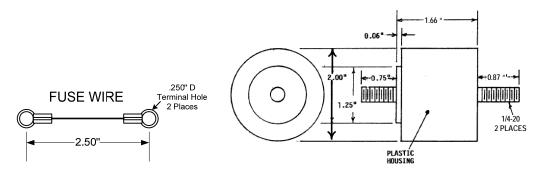
The LPC 11911-124 is a two terminal lightning and surge protective device for protection of electrical and electronic equipment against surges and overvoltage conditions appearing on the "plus" and "minus" lines of the power system. Maximum continuous operating voltage is 1000 VDC.
